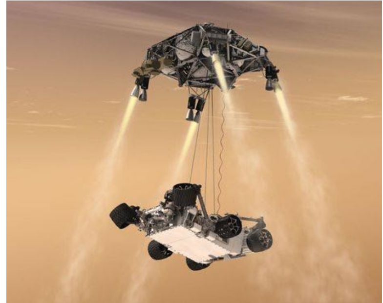
Artist's conception of sky crane lowering Mars rover (Curiosity) to mitigate dust cloud damage to instruments
